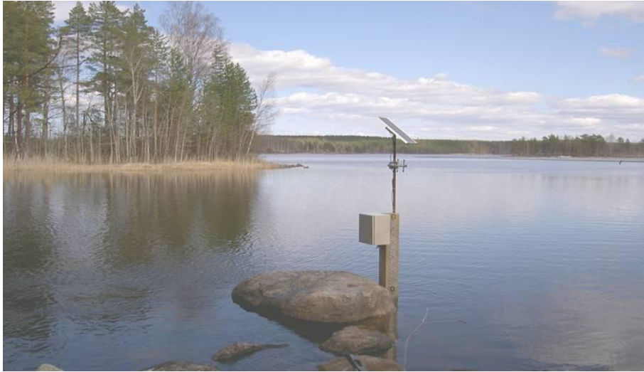
Figure 1. An example of an automated surface water level monitoring station. Photo courtesy of SYKE.
