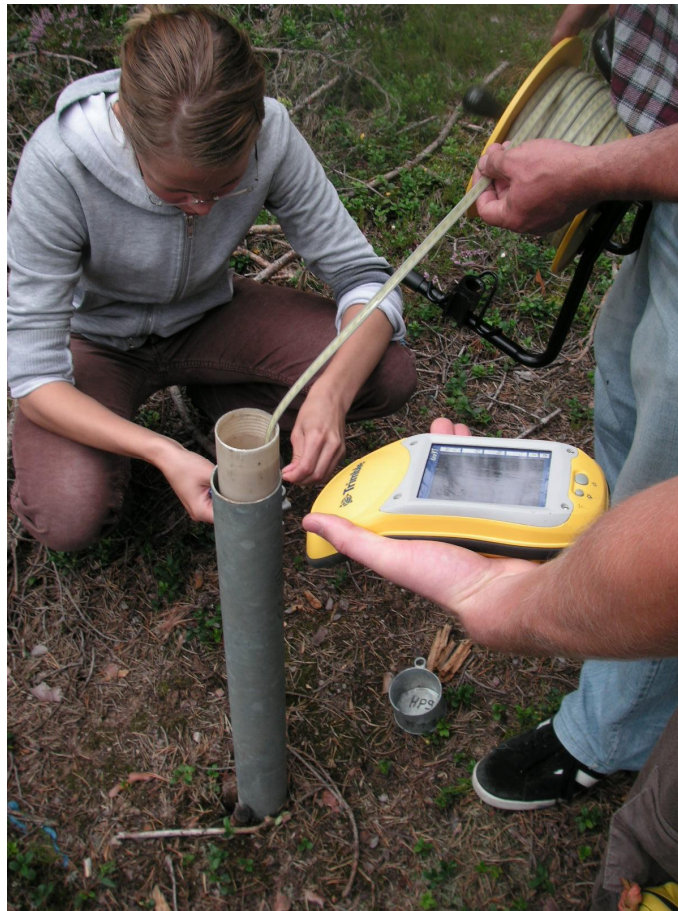
Figure 3. Manual measurement using a tape measure at a groundwater monitoring site. Photo courtesy of SYKE.
