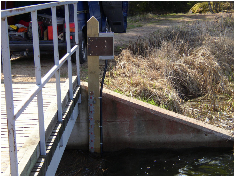
Figure 2. A staff gauge at a water level monitoring site. Photo courtesy of SYKE.
